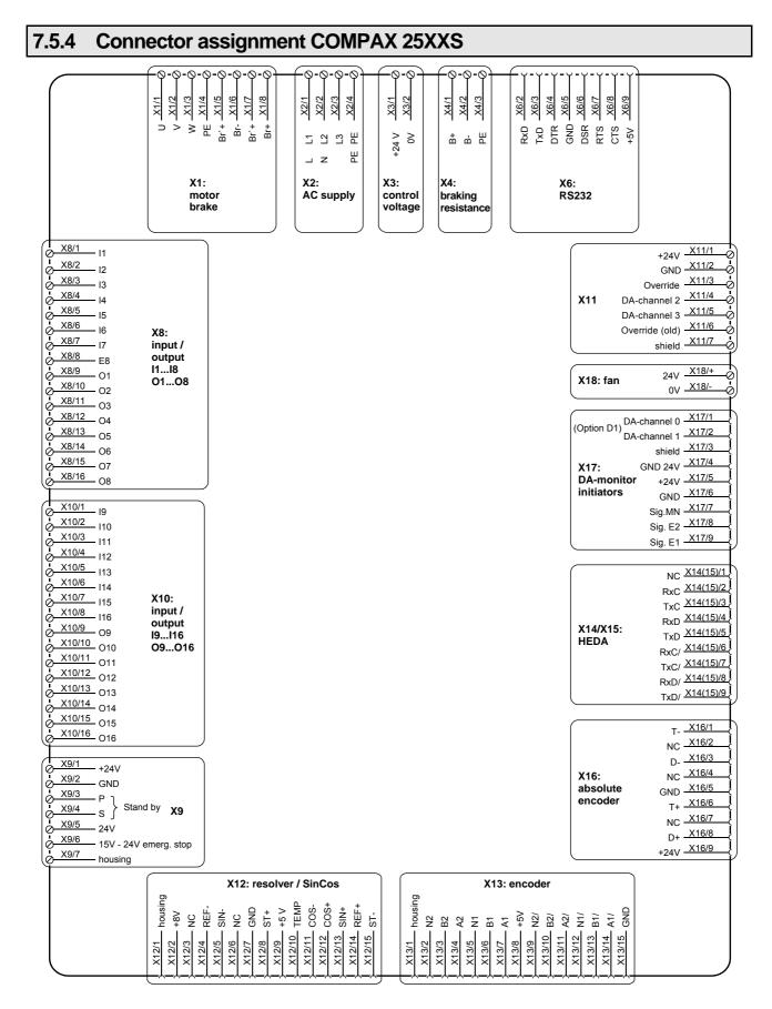
The assignment of X12 does not apply for the S3 option.
